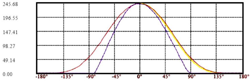
Luminous intensity distribution (unit: cd)
